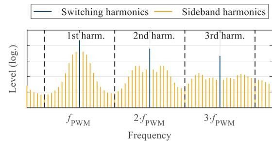
Fig. 4: Typical spectrum of the considered PFC.
