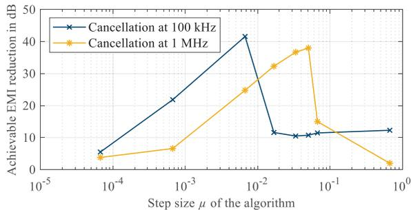
Fig. 7: Investigation of the achievable EMI reduction in respect to the step size  $\mu$  of the algorithm.
