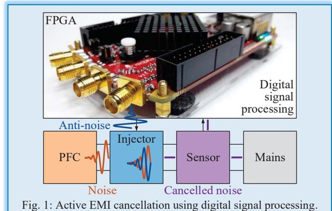
high-frequency electromagnetic interferences (EMI) with significant power levels. This EMI may propagate through the supply lines into the mains and cause disturbances in susceptible systems. To avoid this problem, the conducted EMI is usually attenuated by using passive EMI filters [1]. However, these elements tend to be large, heavy and expensive in comparison to the power electronics itself. Methods of active EMI cancellation can help to resolve this problem.
