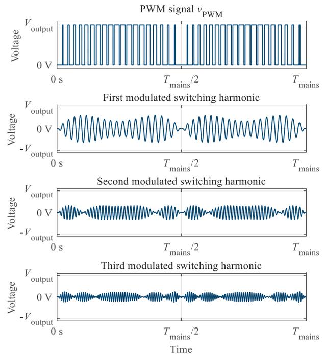
Fig. 3: Typical PWM signal of the considered PFC, modulated switching harmonics.
