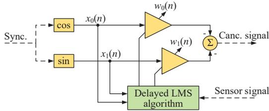
Fig. 6: Single-frequency adaptive notch filter with delayed LMS algorithm.
