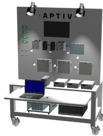
Figure 8 – Planned design of the testbench setup
