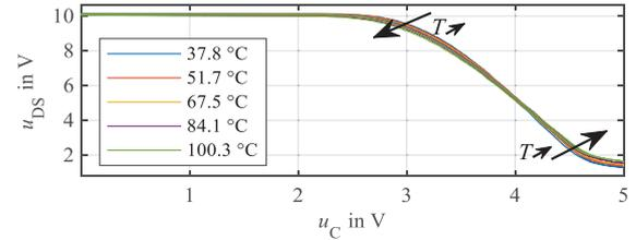
Fig. 11: Transfer characteristic of the MOSFET
