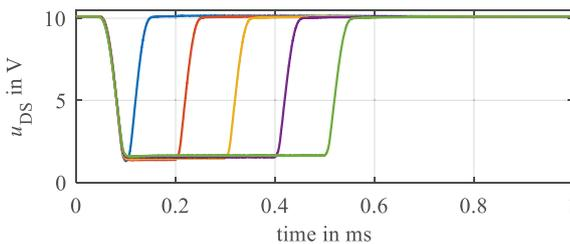
Fig. 10: Measured drain-source voltage  $u_{DS}$
