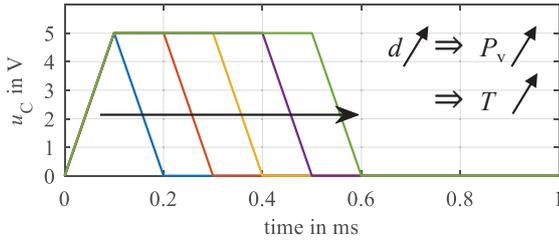
Fig. 9: Test signals to characterize the MOSFET
