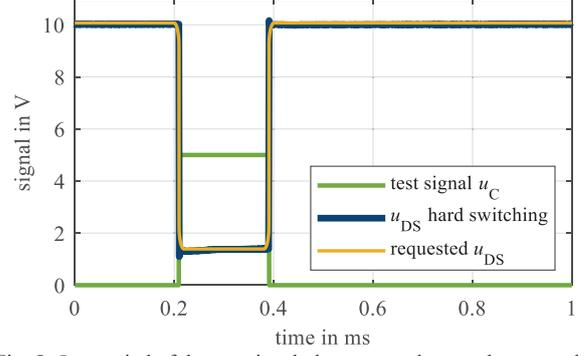
Fig. 5: One period of the test signal, the measured  $u_{DS}$  and requested  $u_{DS}$
