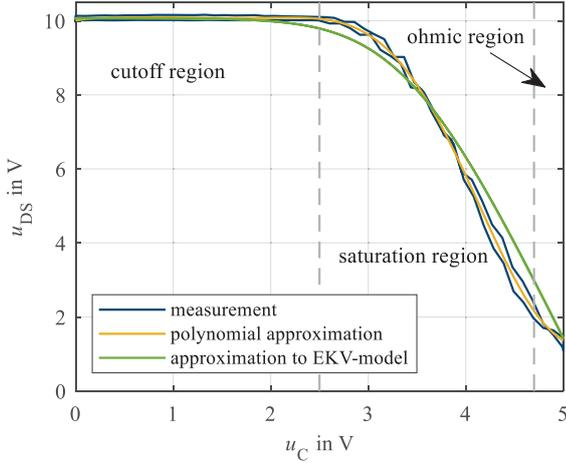
Fig. 6: Measured and approximated system function
