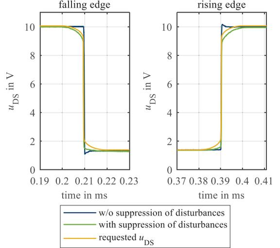
Fig. 8: Measured and requested  $u_{DS}$  (time base refers to Fig. 5) The power losses can be calculated by
