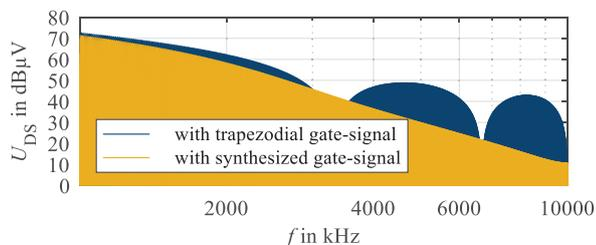
Fig. 13: Simulated  $u_{DS}$  with PWM and synthesized gate-signal
