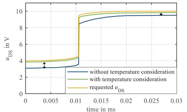
Fig. 12: Measured and requested  $u_{DS}$  respecting the temperature of the MOSFET
