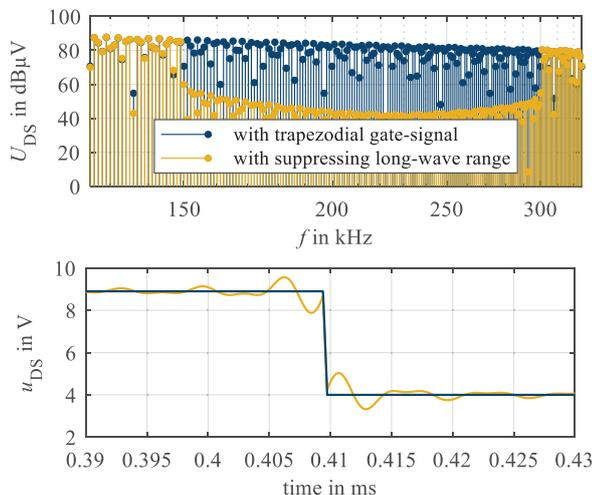
Fig. 14: Simulated  $u_{DS}$  with PWM gate-signal and with suppressing the long-wave range in frequency (top) and time domain (bottom)
