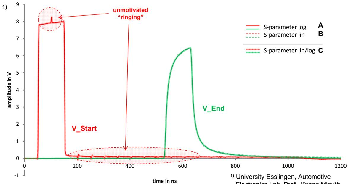
Figure 4: Using S-parameter measurement results in simulation (100 ns bit).
