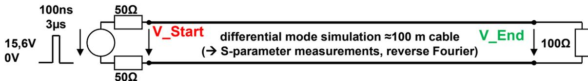
Figure 3: Measurement and simulation set-up (100 ns and 3 μs bit).
