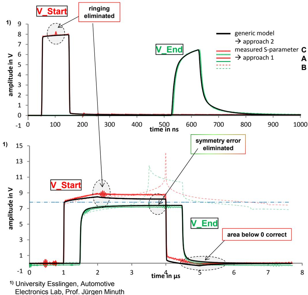
Figure 7: Using S-parameter measurements and approximation results (generic model) in simulation (100 ns and 3 μs bit).
