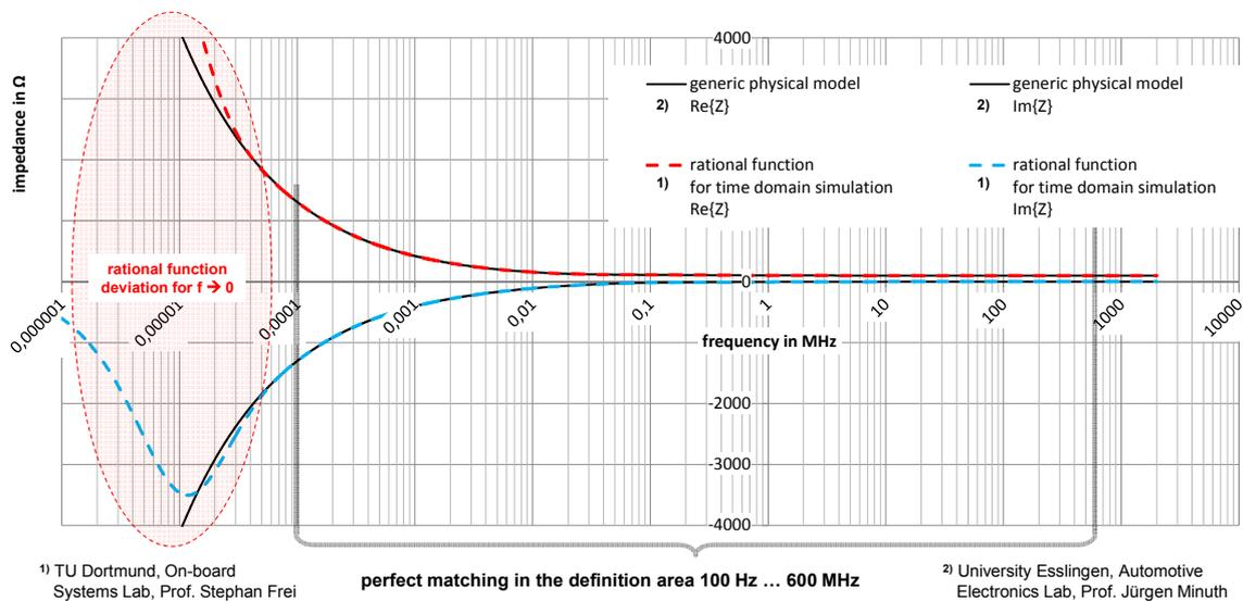
Figure 8: Matching cable impedance  $Z$  “generic model”  $\Leftrightarrow$  “rational function model”.
