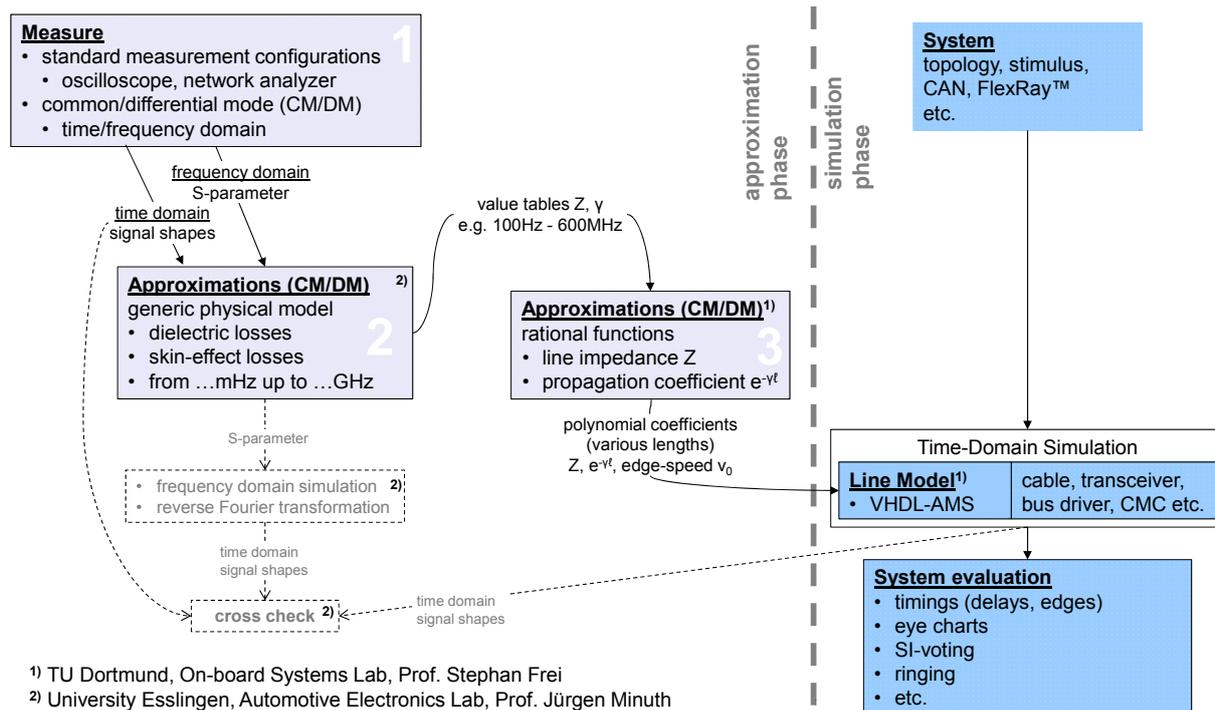
Figure 6: Workflow overview 2<sup>nd</sup> approach “measurement  $\rightarrow$  approximation  $\rightarrow$  simulation”.
