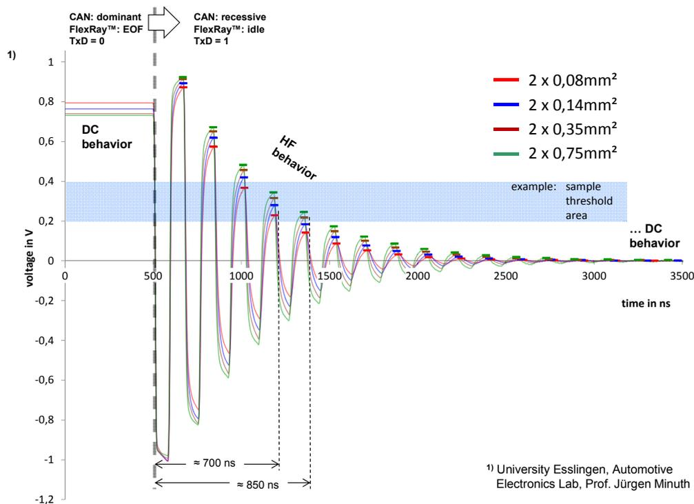
Figure 10: Effect of frequency dependant losses: ringing in CAN and FlexRay™.
