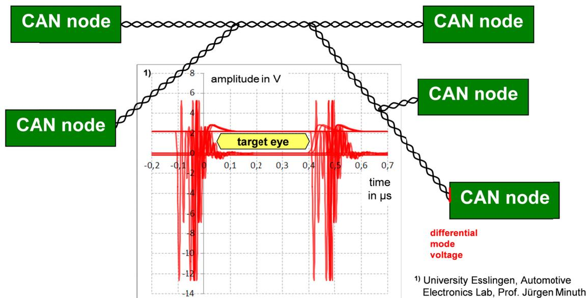
Figure 1: Topology simulation with five CAN nodes at 2 Mbit/sec<sup>1</sup>, the simulation results are superposed to an eye chart.
