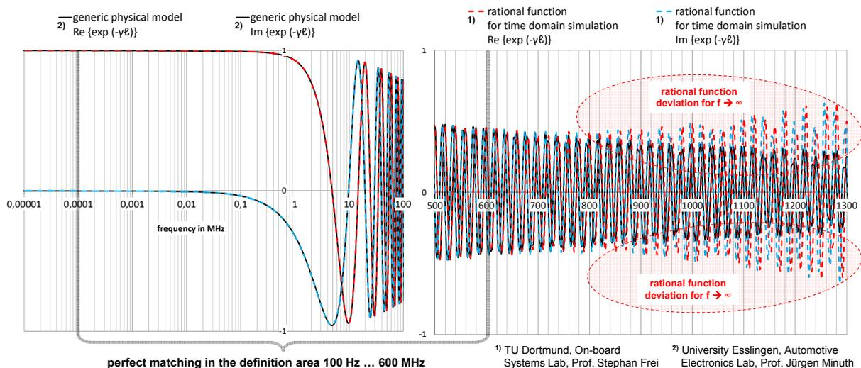
Figure 9: Matching propagation coefficient  $e^{-\gamma \ell}$  “generic model”  $\Leftrightarrow$  “rational function model”.
