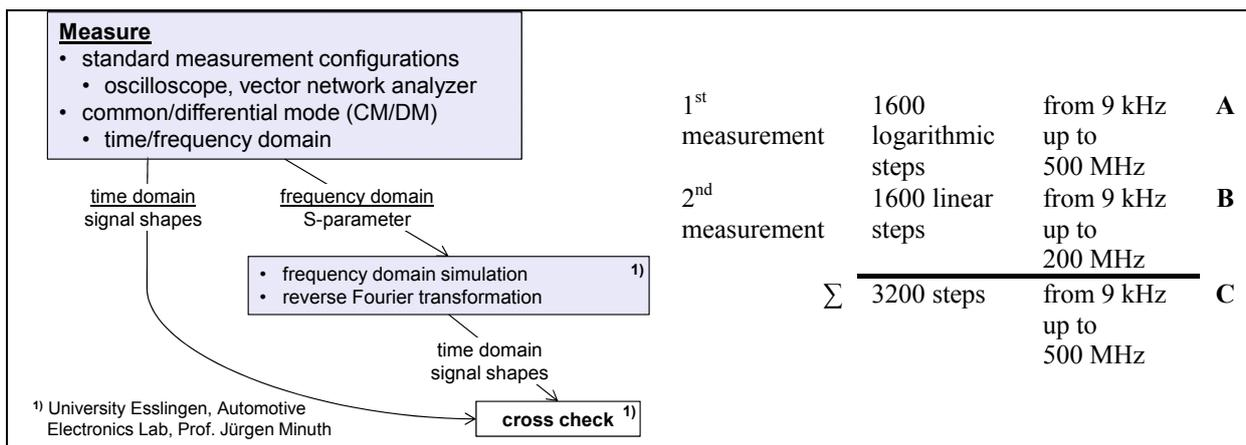
Figure 2: Workflow overview 1<sup>st</sup> approach "measurement → simulation".
