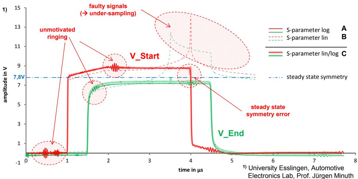
Figure 5: Using S-parameter measurement results in simulation (3  $\mu$ s bit).
