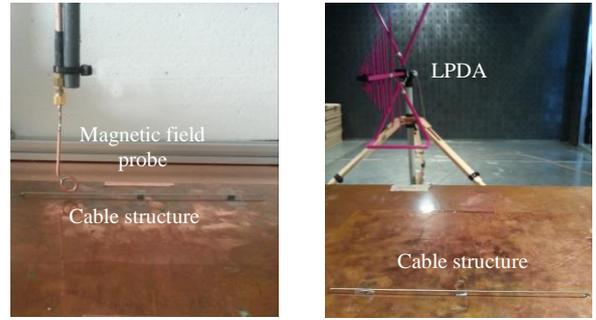
Fig. 14. Near field measurement (left) and antenna measurement (right) of cable structure
