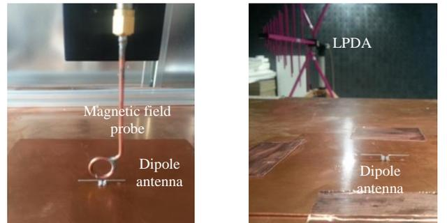
Fig. 11. Near field measurement (left) and vertical polarized antenna measurement (right) of dipole antenna
