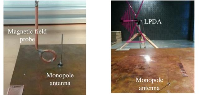
Fig. 10. Near field measurement (left) and vertical polarized antenna measurement (right) of monopole antenna
