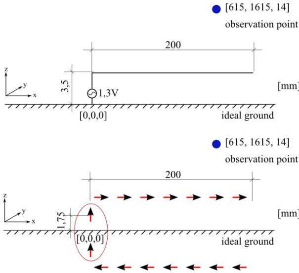
Fig. 8. Approximation of cable structure with Hertzian dipoles
