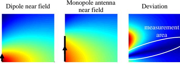
Fig. 5. Comparison of elementary dipole near field and monopole antenna near field
