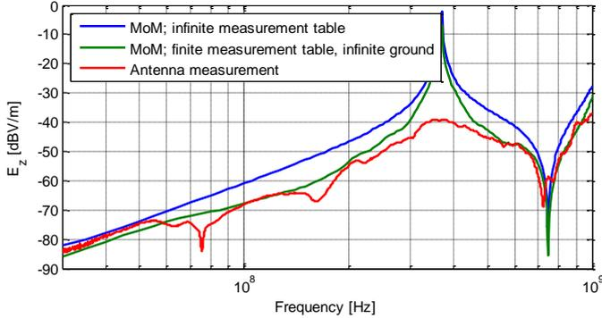
Fig. 2.  $E_z$  of MoM result of radiation from a simple structure above an infinite table and finite table in comparison to real antenna measurement (+ antenna factor from data sheet) in anechoic chamber
