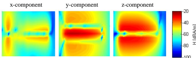
Fig. 13. Near field scans of magnetic field of the structure under test in x-, y- and z-direction at 420 MHz
