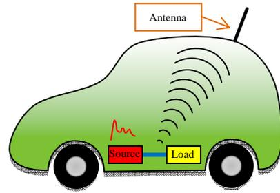
Figure 11. Cable to antenna coupling in vehicle
