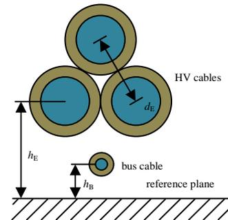
Figure 2. Cross section of the multi conductor line configuration
