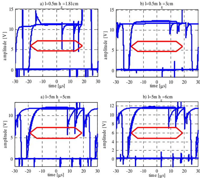
Figure 3. a) broken and b) not effected eye diagrams of the LIN signal
