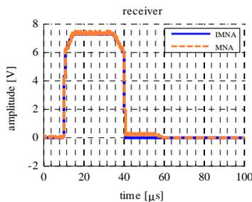
Figure 10. Compare signal at the receiver
