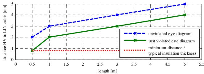
Figure 4. Limits for distances at parallel lengths of HV and LIN cables
