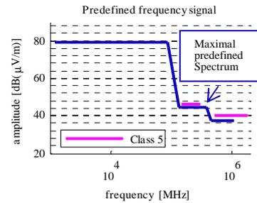
Figure 12. Antenna signal amplitude in frequency domain
