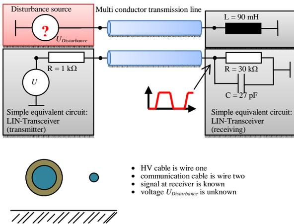
Figure 8. HV cable and LIN communication cable
