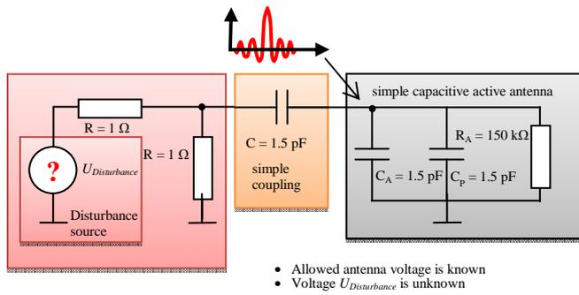
Figure 14. Equivalent circuit for cable antenna coupling in low frequency range
